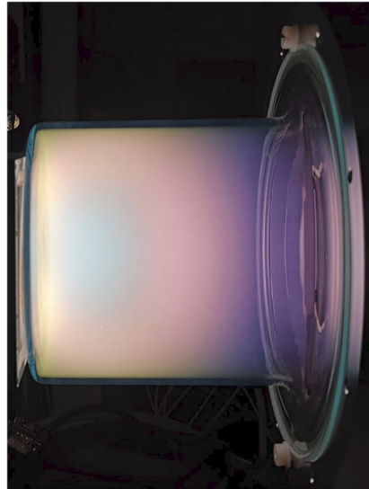
Figure 3. Photograph of a low-pressure iodine plasma produced in the PEGASES thruster prototype. Reproduced with permission from [26].
