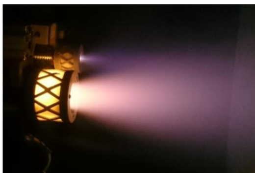
Figure 40. Photograph of the BIT-3 ion thruster (bottom discharge) and BRFC-1 RF neutralizer (top discharge) operating with iodine. From [233]. Reprinted by permission of the American Institute of Aeronautics and Astronautics, Inc.
