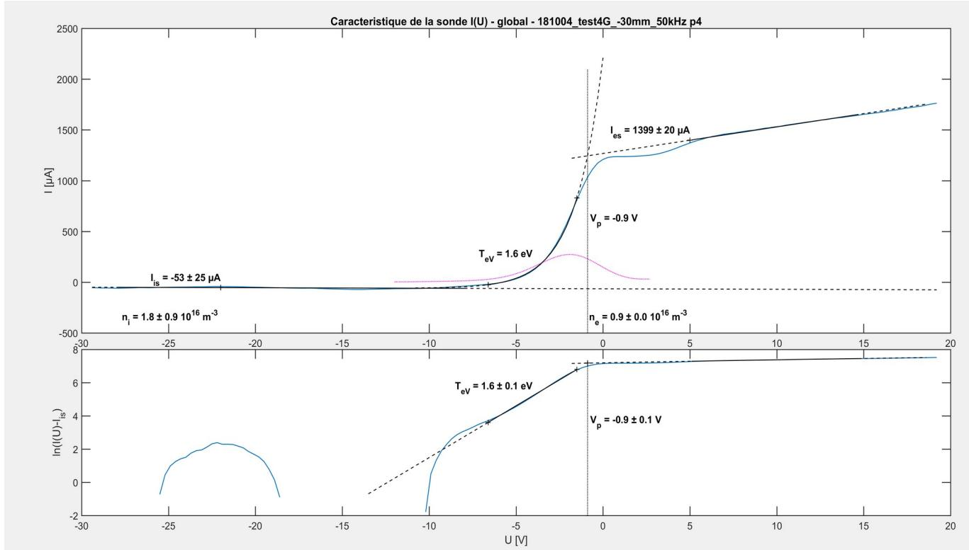
As expected, the (positive) electron current is stronger than the ion current.
