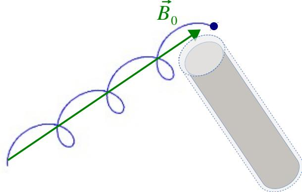
The probe surface perpendicular is a rectangle of length  $l_L$  and width  $2\rho_L$ . The probe can be reached from both sides. The probe collection area in the direction of the field is for this configuration:
