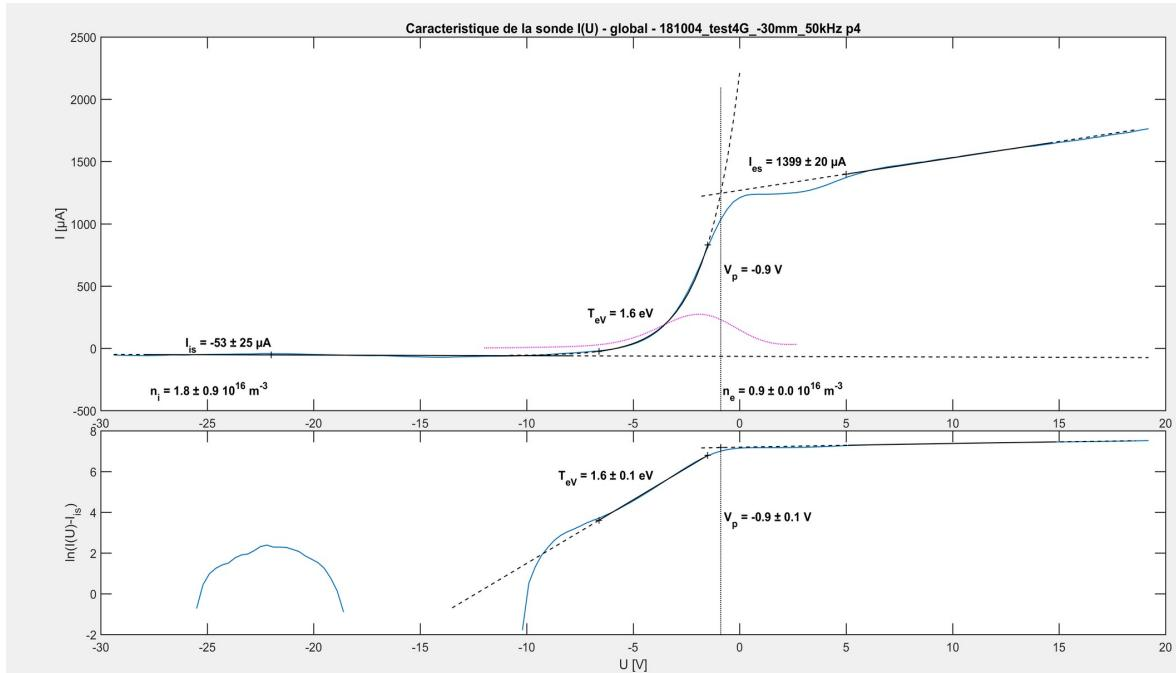
The first graph represents the current as a function of the polarization voltage :  $I(U_L)$ .
