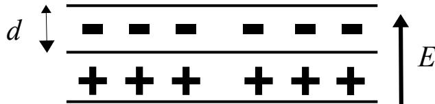
We consider a plasma composed of positive (ions) and negative (electrons) opposite charges of the same density  $n_i = n_e$ . We assume a plane charge separation at a depth  $d$  between both species.
