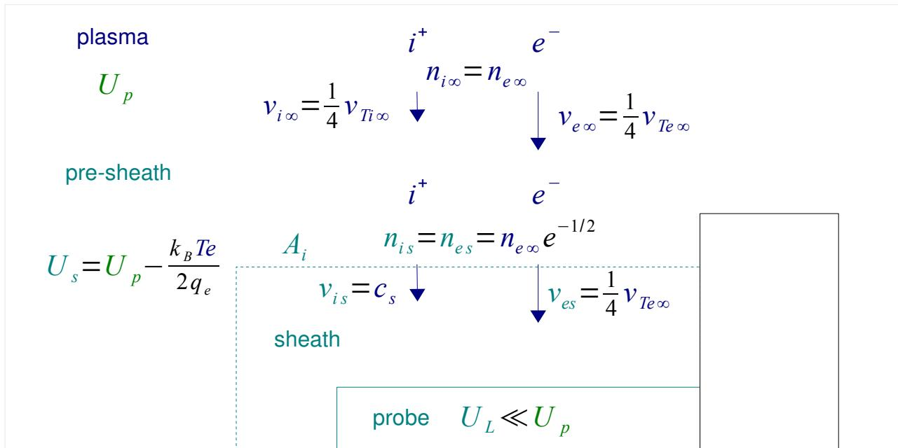
The plasma ion thermal velocity is lower than this velocity (because their mass is much larger and their temperature is lower than the electron ones). Around the sheath, in a zone called pre-sheath, they undergo a first electric acceleration towards the sheath. The acceleration is provided by a potential difference between the plasma core  $U_p$  and the sheath surface :
