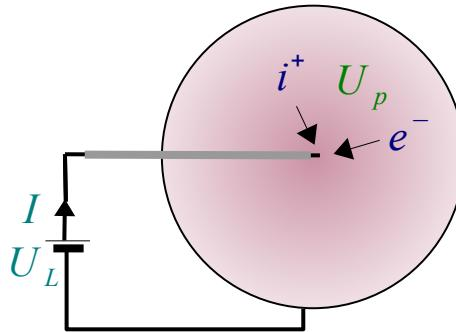
Since the Langmuir probe potential  $U_L$  is different from the plasma potential  $U_p$ , the probe has a different effect on the plasma electrons and ions. Because of the potential difference, over a certain distance around the probe, the quasi-neutrality of the plasma is no longer verified: it is the sheath that surrounds the probe. If the probe potential is lower than that of the plasma, the sheath mainly consists of ions. Electrons dominate in the opposite case.
