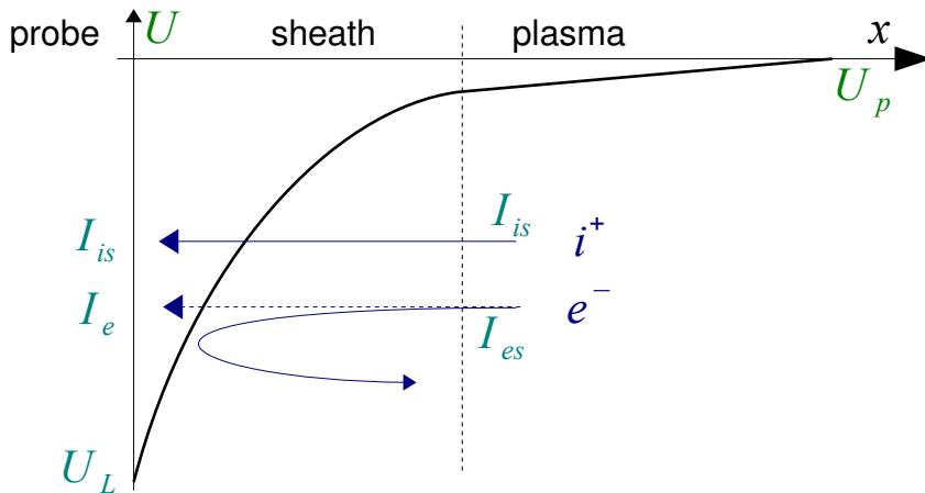
The ions are attracted by the probe: all the ions at the entrance of the sheath reach the probe, the ion probe current  $I_i$  is the ion saturation current  $I_{is}$  :
