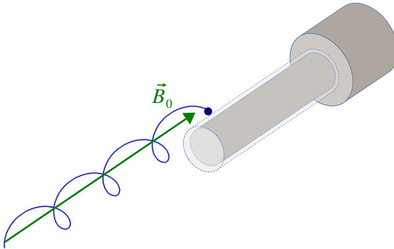
For the ion collection, the collection area includes the probe surface:
