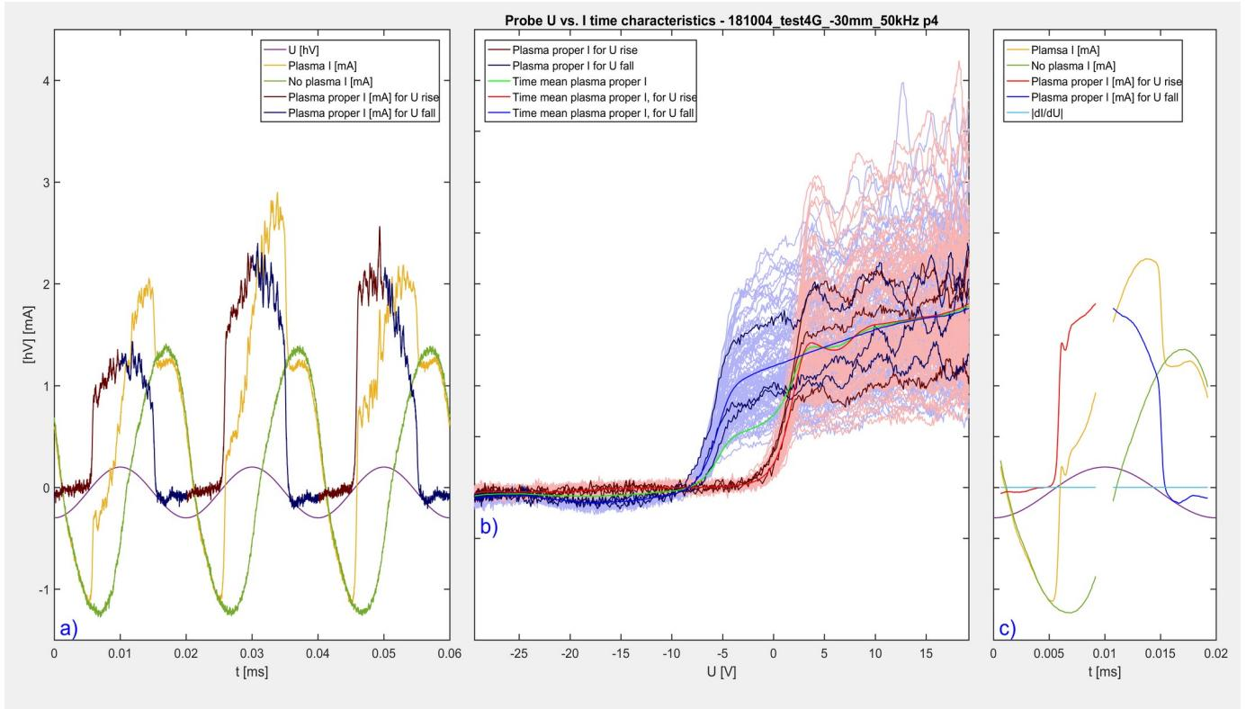
The graph a) shows time signals during 3 generator periods. The yellow plot corresponds to the probe current (in  $\text{mA}$ ). The sinusoidal signal in purple plot shows the generator signal (in  $\text{hV}$ ). The current signal is very asymmetrical with respect to the generator signal. However, the current response of the plasma should mainly depend on the polarization voltage.
