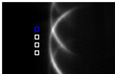
It is possible to analyze the vertical wave propagation the same way it is done with the probe by selecting 2 pixels vertically separated by several millimeters.
