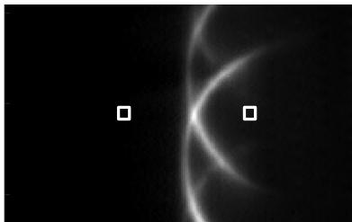
Compute the cross-correlation between 2 pixels radially spaced on each side of the filament at the probe height with and without the vertical magnetic field. Each pixel will be 8 mm away from the filament.
