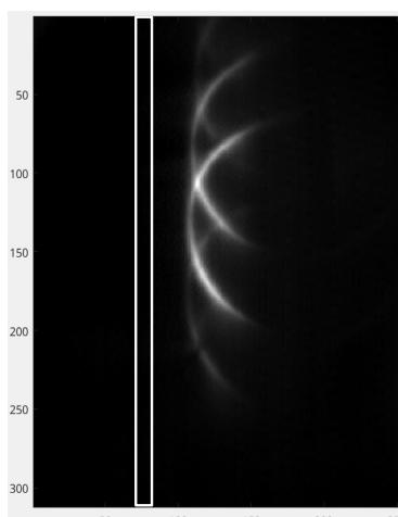
The pixel image allows to do a more complete analysis using all pixels in the vertical direction to obtain a  $k_y, \omega$  dispersion relation for the HFS gradient zone for a radial position. We choose the same pixel radial position in the HFS gradient zone  $ix_g$ .
