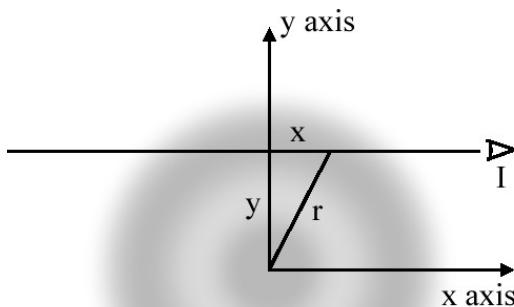
$f_2$  is the local emitted light for each position in the plasma  $(x, y)$  in a horizontal plane.  $F$  is deduced from  $f_2$  by integration:
