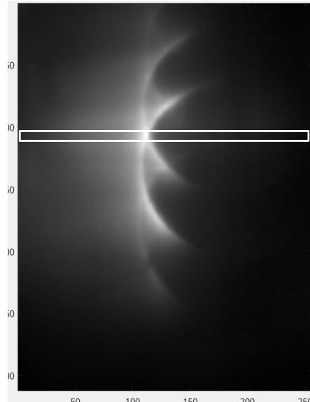
We also need a reference position. We assume the position for which the light is maximum corresponds to the position for which the electron density is maximum.
